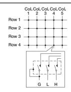
Each crosspoint in the matrix consists of a 3-pole Form A (normally open) relay. The shield of each relay is connected to the column GUARD line.
